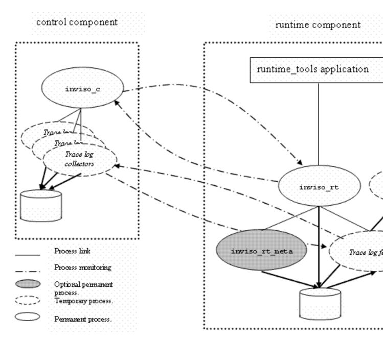
Figure 1.1: Inviso Trace System Architecture Overview.
