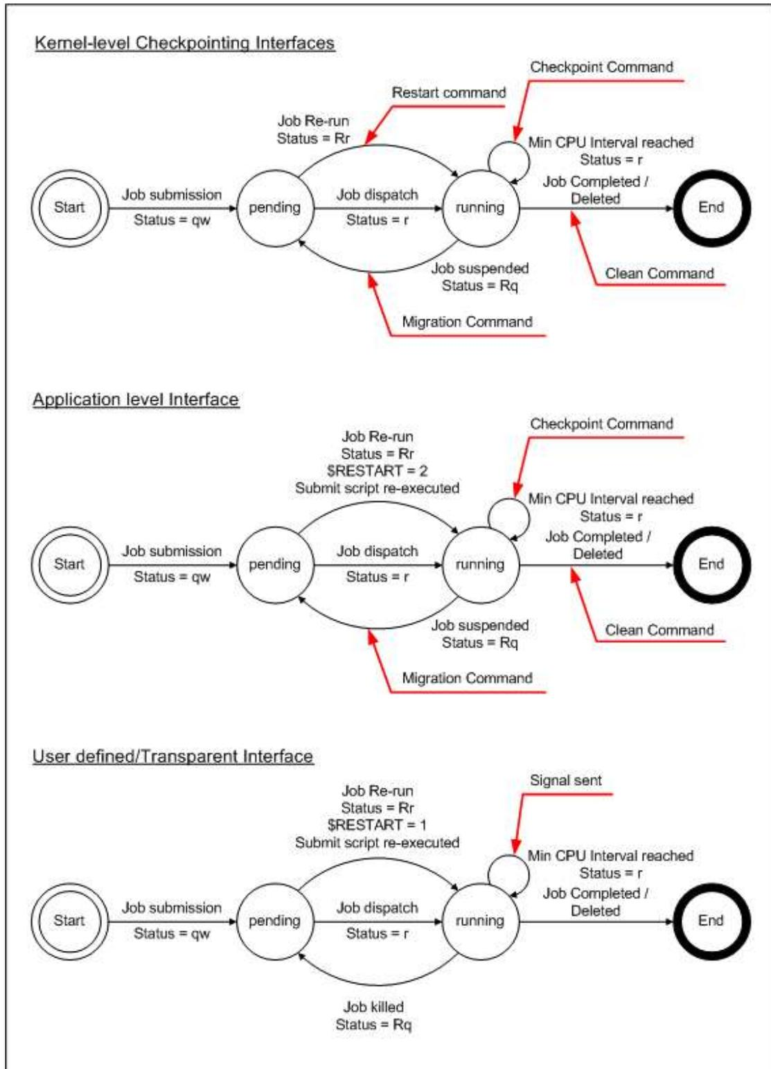
Illustration 2 State diagram of the different interfaces
